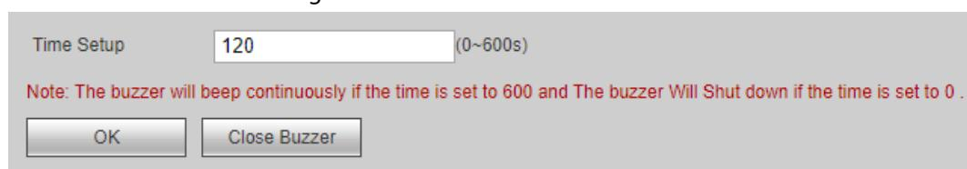
Step 3 Set the time for the buzzer alarm.
